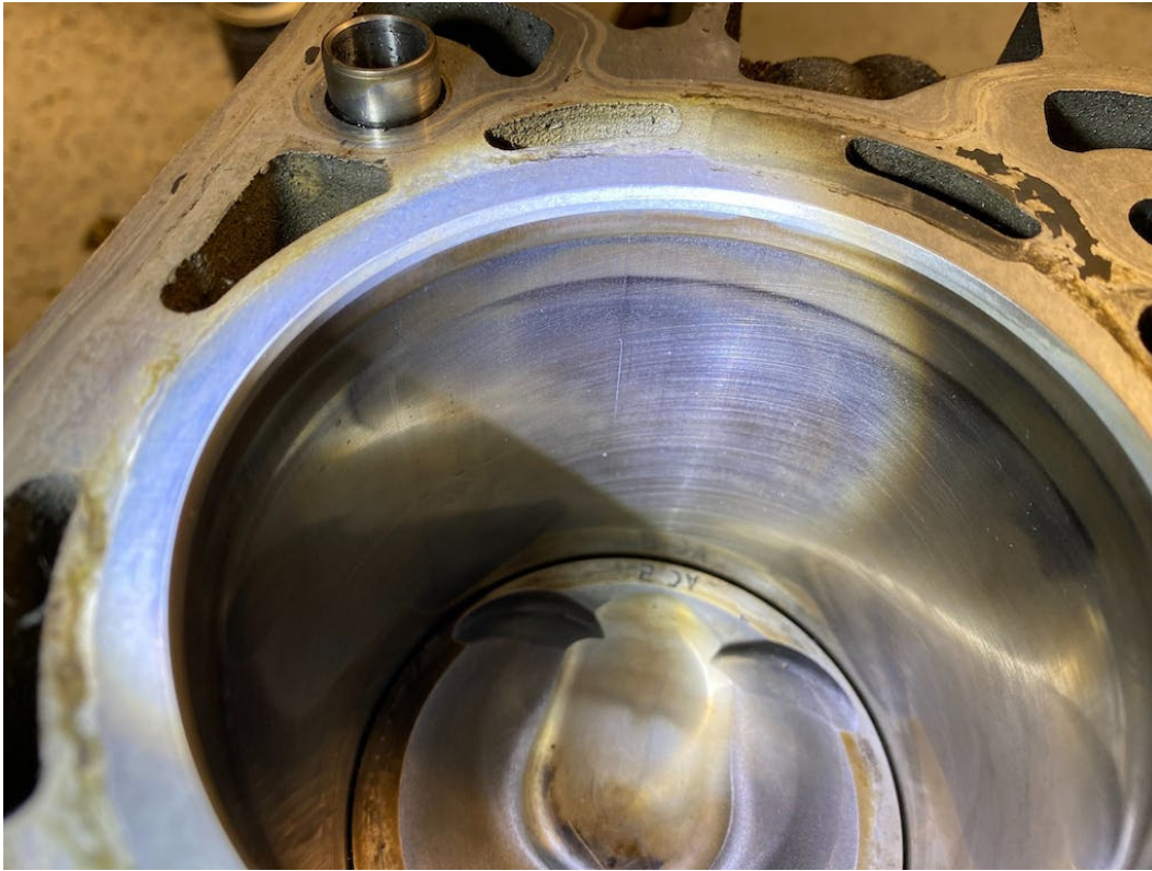
Scratched cylinder wall due to broken ringland and rings on piston. Bozi Tatarevic
